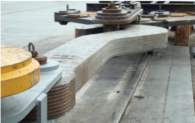
150 ton load test of a custom-built anchor chain jack
