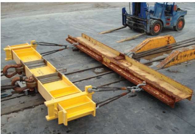
235 ton load test of a 20 ft. (yellow) turbine-lifting spreader beam
